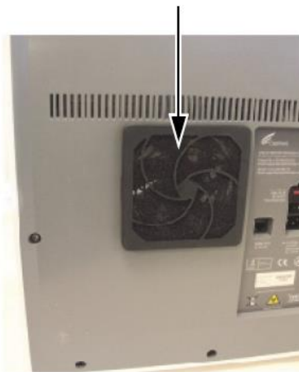
Filter and Fan Guard Installed
